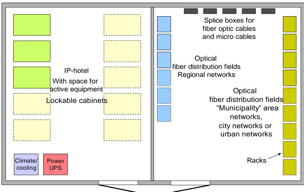
Figure 6: Node with multiple operators
